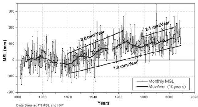
Figure 1. Complete (1882-2008) monthly average time series of sea level at Cascais tide gauge with a 10-year moving average superimposed.
