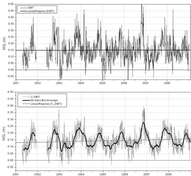
Figure 2. a) Raw daily Mean Tide; b) corrected daily Mean Tide by the inverse barometric effect and the respective 60-days moving average (regression lines are shown in both graphs).
